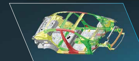
Reinforced Body Structure with Hot Press Formed Steel
